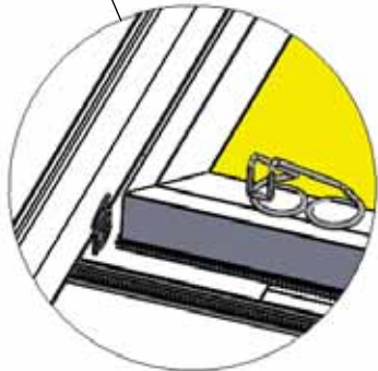
Gusset Clip and Wire Safety Clip Installed on the inner corner of the Claro T panel edge (as shown)
